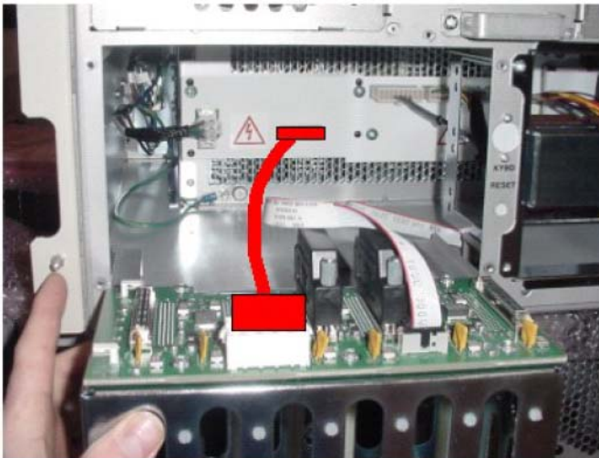
Figure 20: SCSI power cable attached to T board
