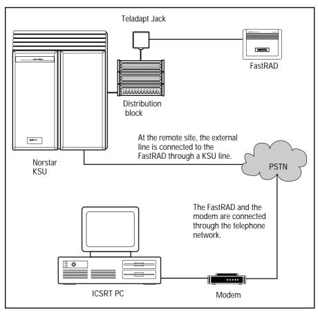
Figure 1 – System overview of remote connection
