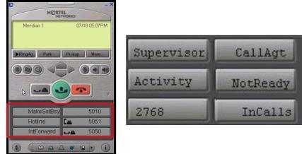
The DN/Feature Tray contains the Primary User Interface controls plus six feature keys. An additional six features are accessed with the **Shift** key.
