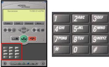
The Number Pad Tray contains the Primary User Interface controls plus a keypad. The numeric keypad mimics a regular phone's dialpad.
