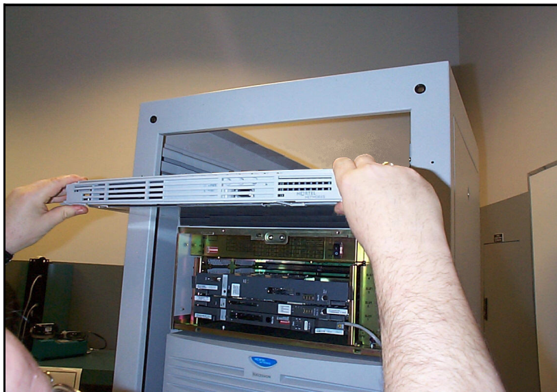
Figure 20 Rack-mounting the Succession Signaling Server
