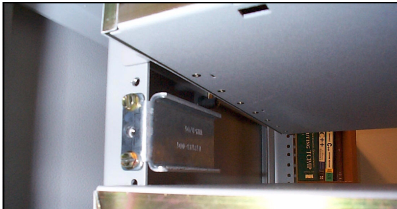
Figure 10 Installed rack-mount bracket
