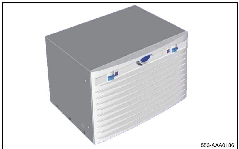
Figure 2 Branch Office H.323 WAN Gateway/H.323 WAN Gateway Expansion chassis
