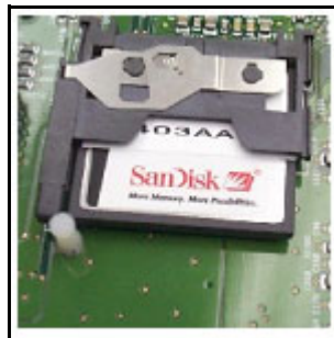
Figure 13 Retaining pin fully inserted
