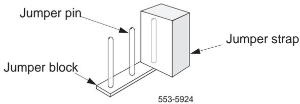
**Note 2:** Jumper blocks labelled P1,P2, P28-P34 are used for testing and future options only and all straps associated with the "P" labelled jumper blocks are open at all times.
