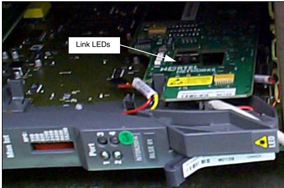
Figure 7 Succession Media Gateway SSC IP daughterboard link LED
