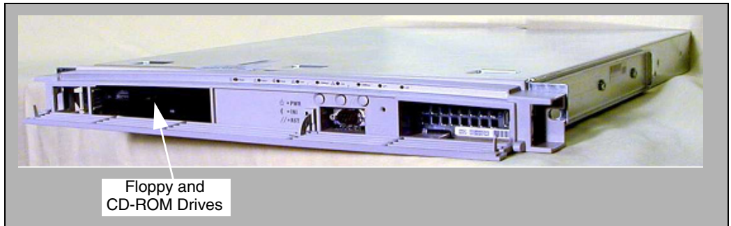
Figure 14 Succession Signaling Server with open bezel door
