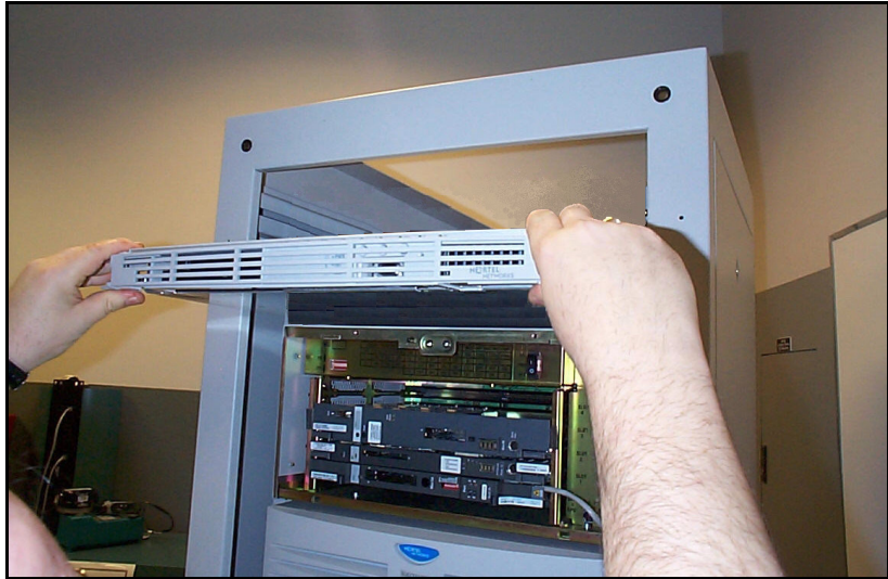
Figure 10 Rack-mounting the Succession Signaling Server
