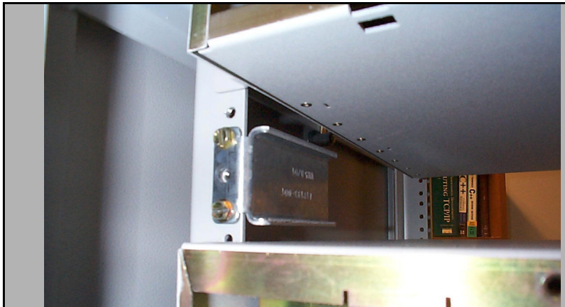
Figure 29 Installed rackmount bracket
