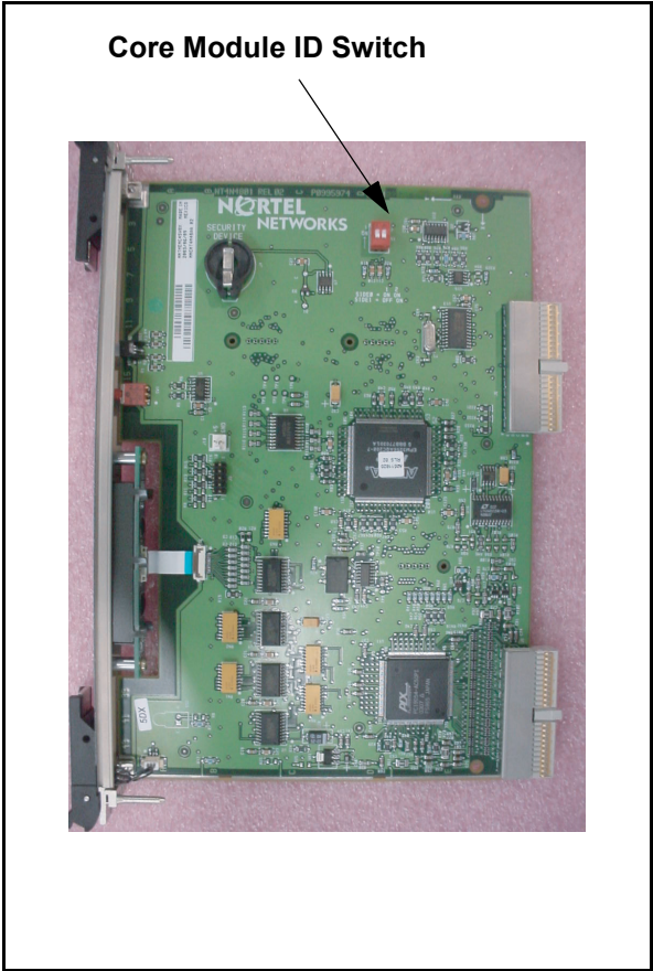
Figure 91 Core Module ID switch
