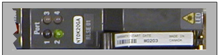
Figure 63 SSC faceplate Succession Call Server to Succession Media Gateways Port LEDs
