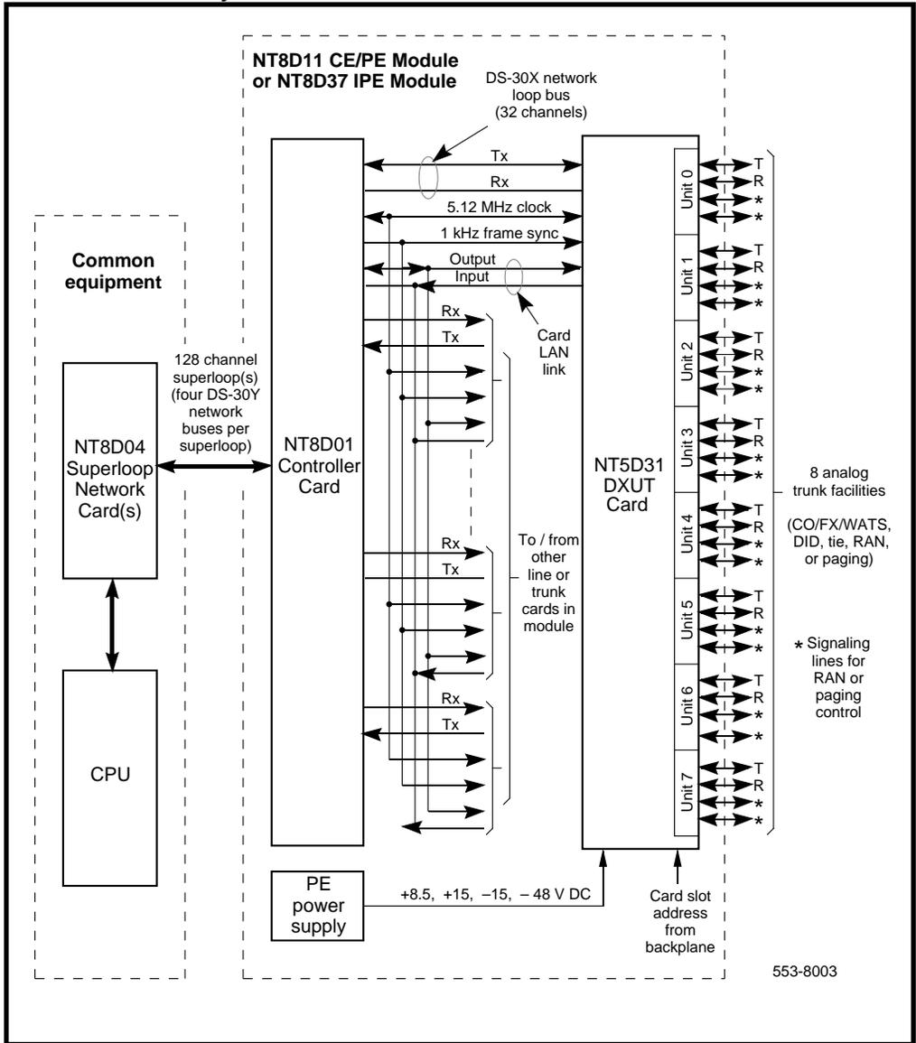
DS-30Y network loops extend between controller cards and superloop network cards in the CE and function in a manner similar to DS-30X loops. Essentially, a DS-30Y loop carries the PCM timeslot traffic of a DS-30X loop. Four DS-30Y network loops form a *superloop* with a capacity of 128 channels (120 usable timeslots). Various superloop configurations exist. See *Meridian 1 system engineering* for more information on superloops.
