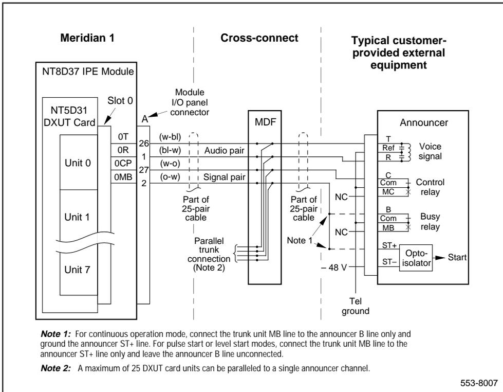
**Note:** The “B” (busy) signal line shown in Figure 25 (not represented in Figure 26) is used to indicate availability of an announcement machine message to the trunk unit when configured for the continuous operation mode. This signal is made active (ground) by the announcement machine if the channel contains a recorded message and is in an on-line condition. The “B” line is not connected to a trunk unit when configured for start mode operation.
