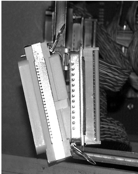
Figure 4 Disconnect filter from backplane cable
