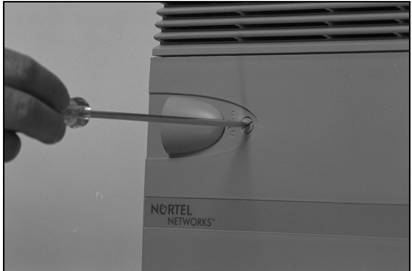
Figure 35 Unlocking the latches
