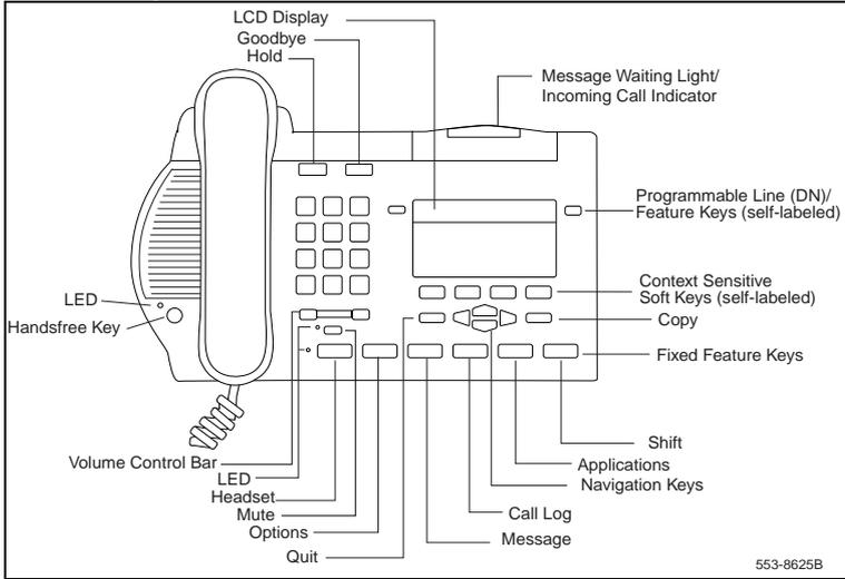
The **M3904** has six Programmable Line (DN)/Feature Keys (self-labeled), with two features or lines (DNs) configured on each key. The **M3904** also has four Context Sensitive Soft Keys (self-labeled).
