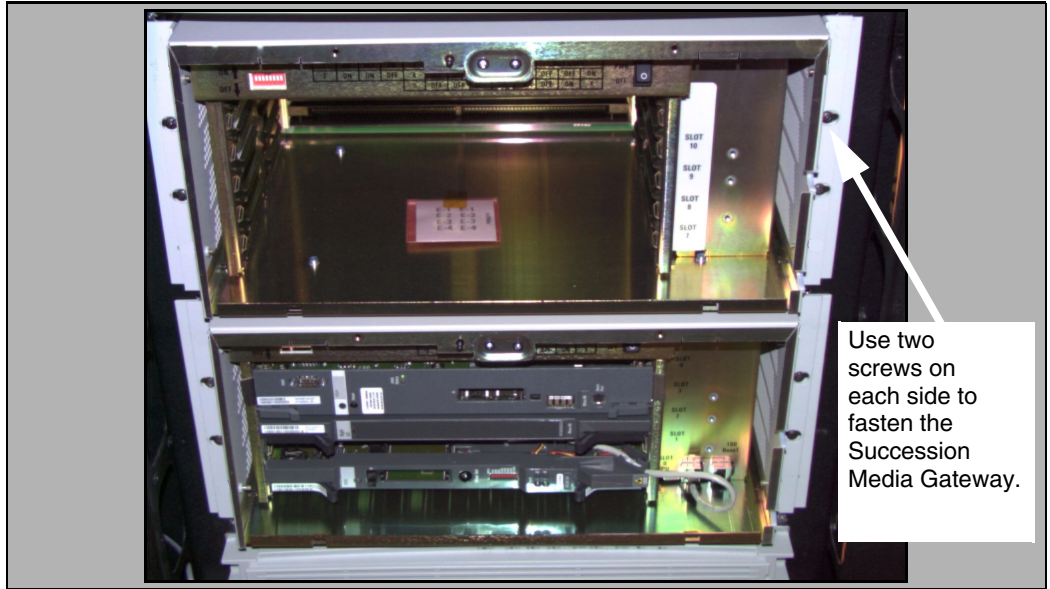
Figure 23 Succession Media Gateway installed in a rack
