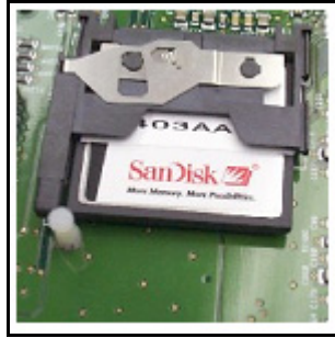
Figure 106 Retaining Pin fully inserted
