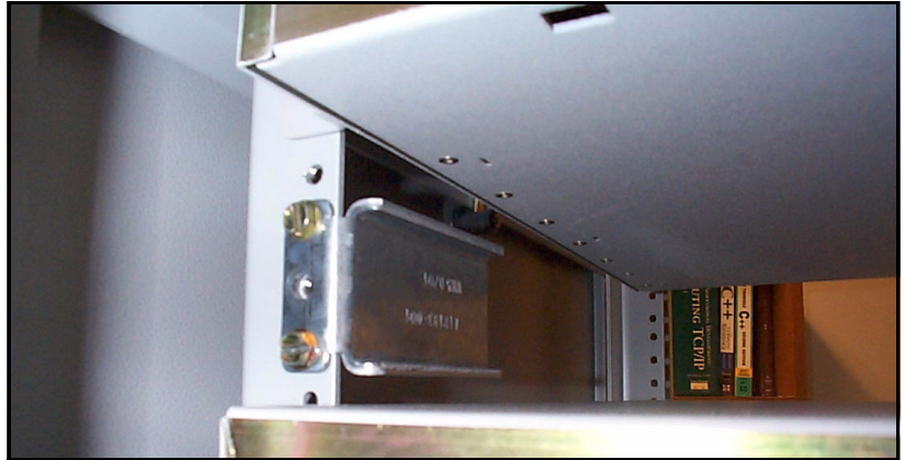
Installed rack-mount bracket
