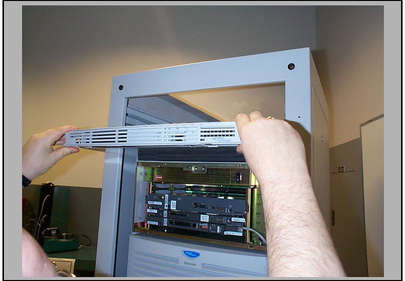
Figure 30 Rackmounting the Succession Signaling Server
