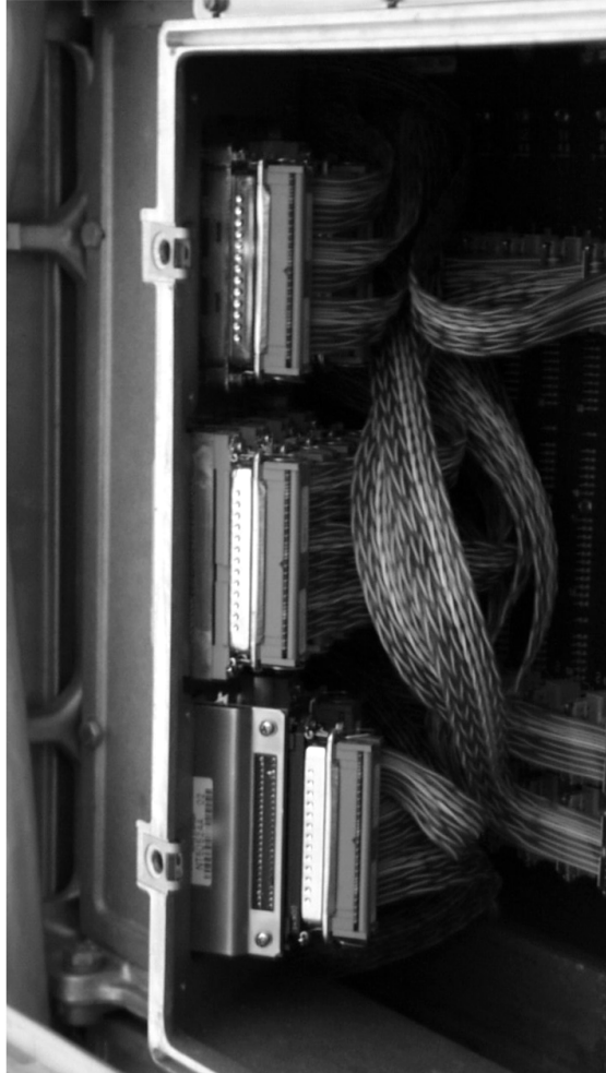
Figure 5 Install adapter 50-pin connector in backplane 50-pin cable connector
