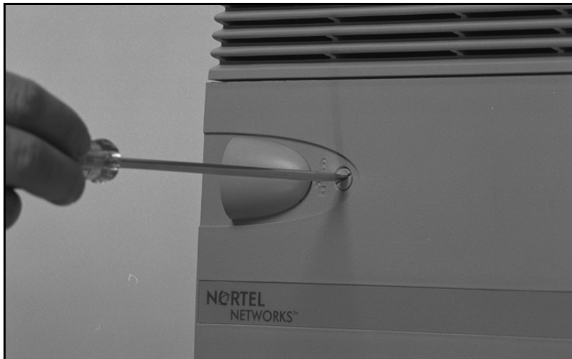
Figure 29 Unlocking the latches
