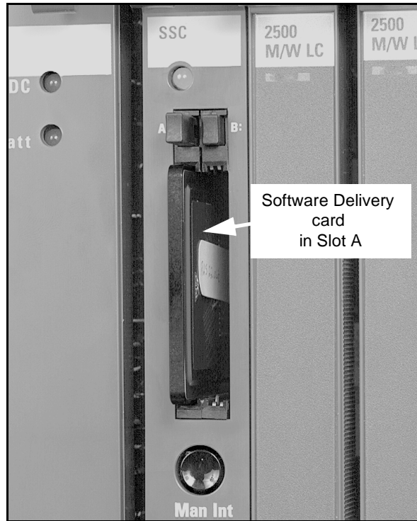
Figure 58 PCMCIA card slot location
