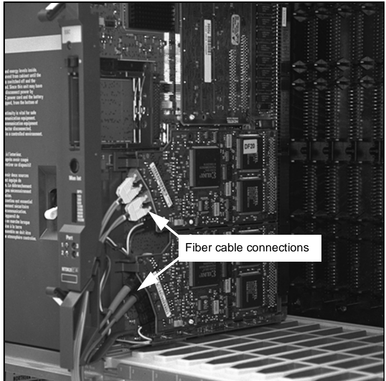
Figure 14 Fiber-optic cable connections
