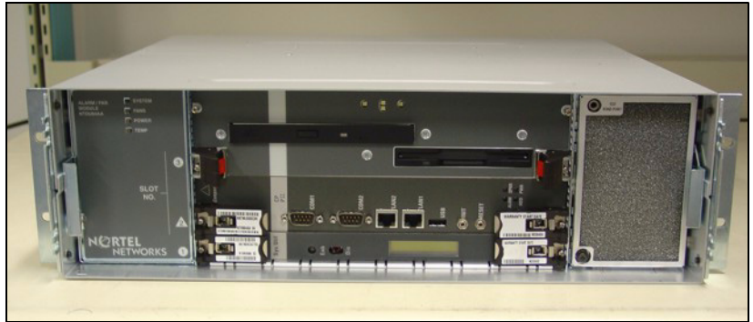
Figure 13 CS 1000E Call Server with installed ear brackets
