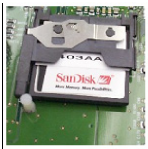
Figure 112 Retaining Pin fully inserted
