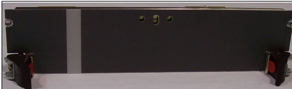
Figure 21 CS 1000E CP PIV Drive Carrier Card blank faceplate replacement
