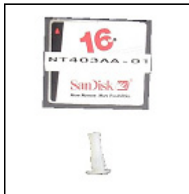
Figure 106 CompactFlash card and Retaining Pin
