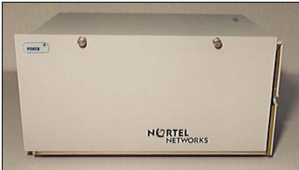
Figure 33 Fitting the front faceplate on the chassis
