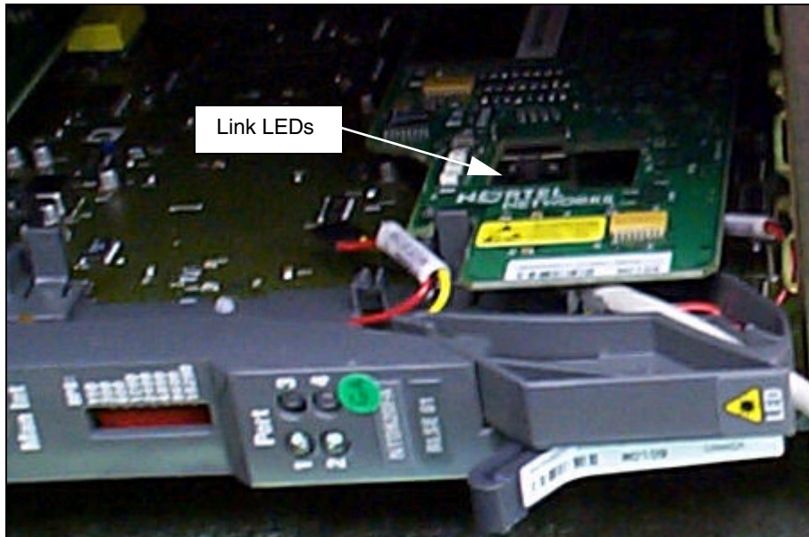
Figure 7 MG 1000S SSC IP daughterboard link LED
