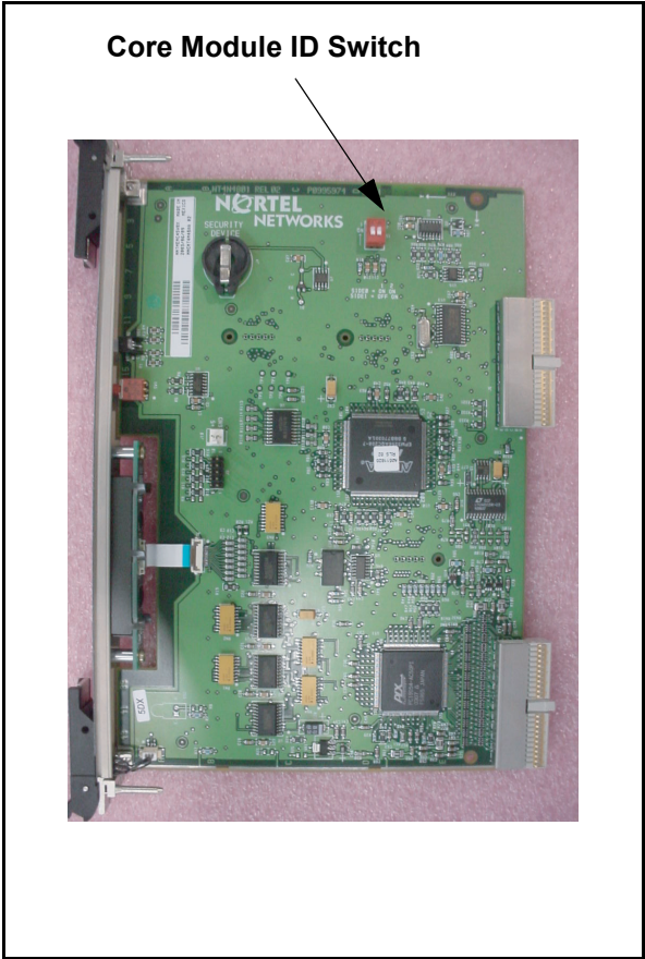
Figure 41 Core Module ID switch
