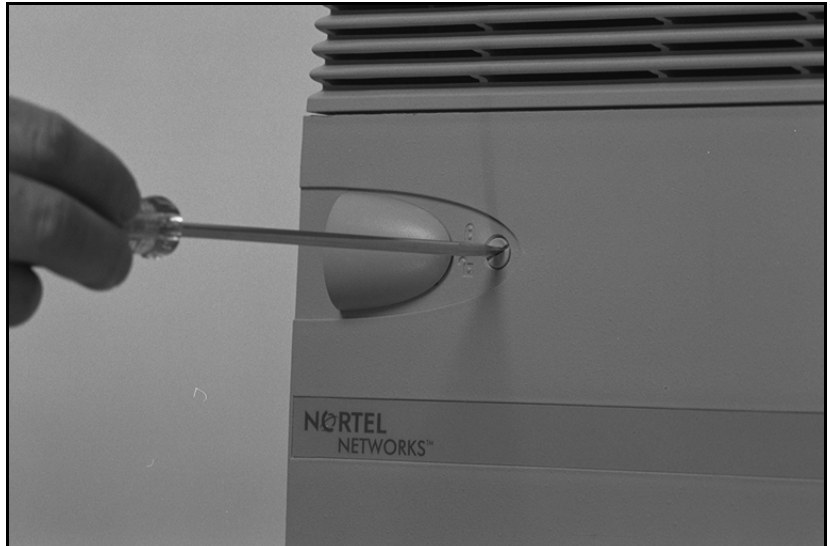
Figure 36 Unlocking the latches
