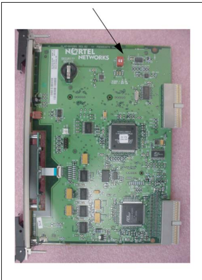
Figure 6 Core Module ID switch
