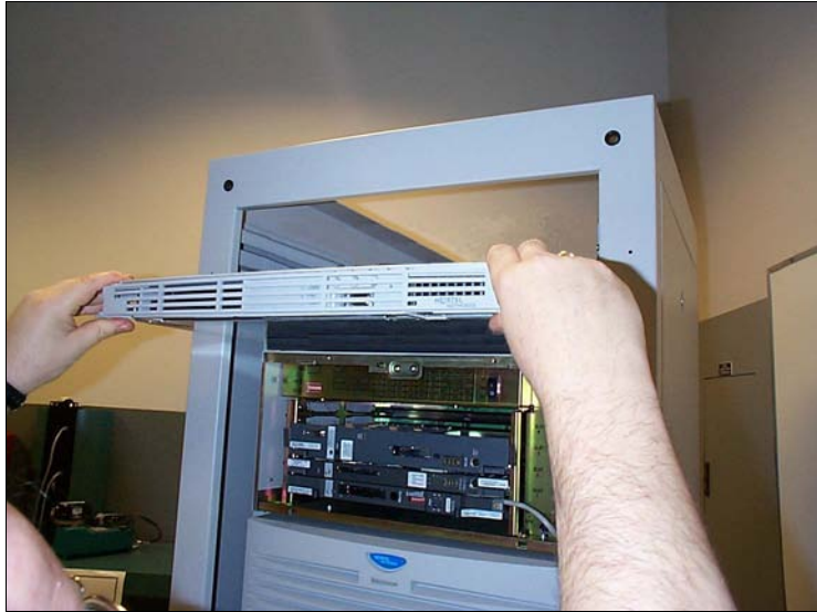
Figure 25 Rack-mounting the Signaling Server
