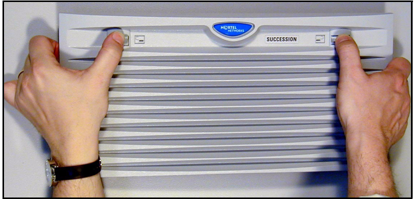
Figure 10 Depressing latches and pulling back on front cover
