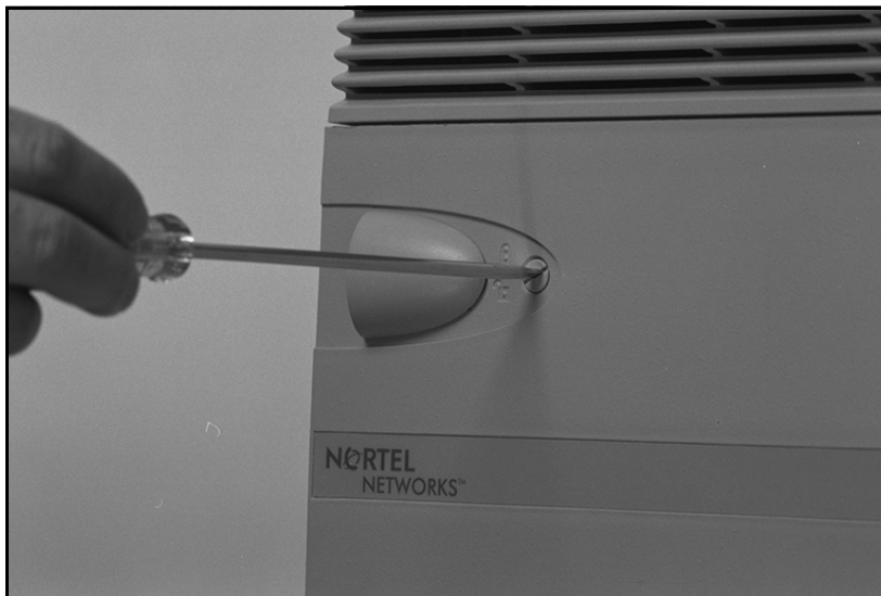
Figure 38 Unlocking the latches
