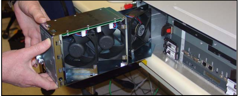
Figure 13 Alarm/fan module
