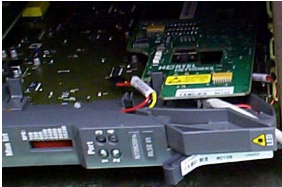
Figure 10 Media Gateway SSC IP daughterboard link LED
