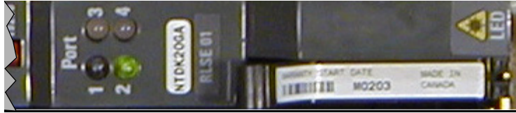
Figure 95 Media Gateways SSC faceplate Port LEDs
