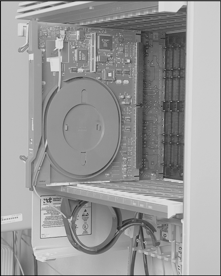
Figure 26 Fiber Receiver card in fiber Expansion Cabinet (NTDK23 shown)
