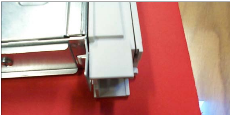
Figure 23 Snapped-in bezel door
