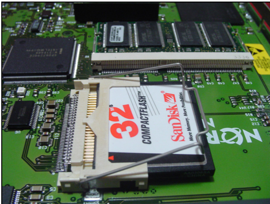
Figure 265 Lift the metal clip on the CompactFlash card
