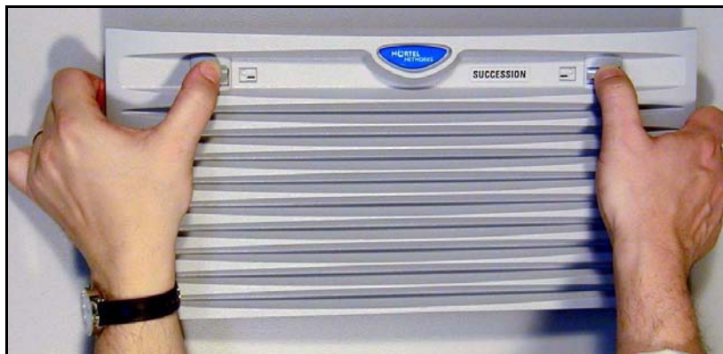
Figure 17 Depressing latches and pulling back on front cover
